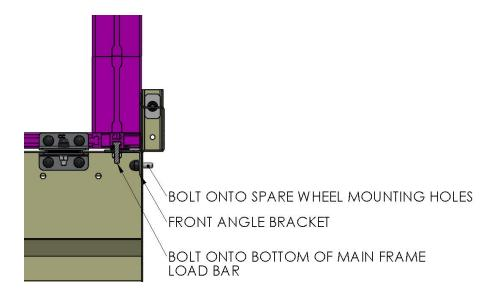
**NB!** The Canopy Camper must rest solely on the mounting brackets and no load is allowed on the load bin. Once this is completed, the Canopy Camper has been installed successfully.
