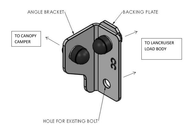
The image below shows the mounting bracket position on DC, the SC position is slightly offset.
