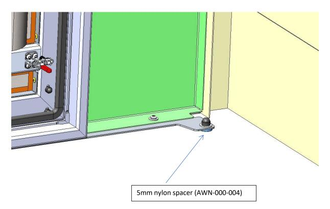
The 5mm spacer (AWN-000-004) elevates the filler panel and creates a  $\pm\,5$ mm gap between the load bin and camper which is sealed with the supplied D-Rubber
