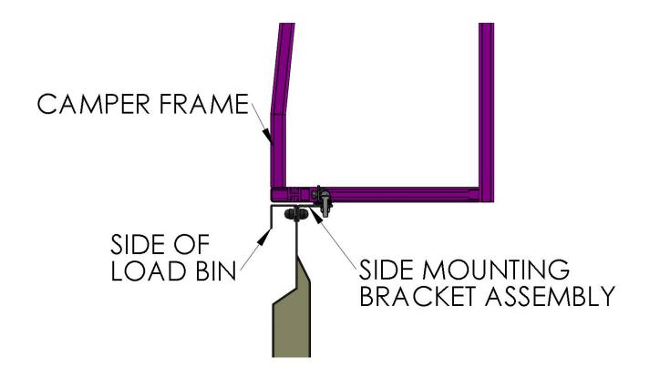
Side Mounting Bracket assembly with fasteners supplied. 6 sets for the DC and 8 sets for the SC.
