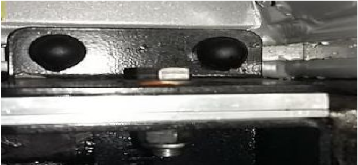
Figure 19: Front Support Bracket Installed
