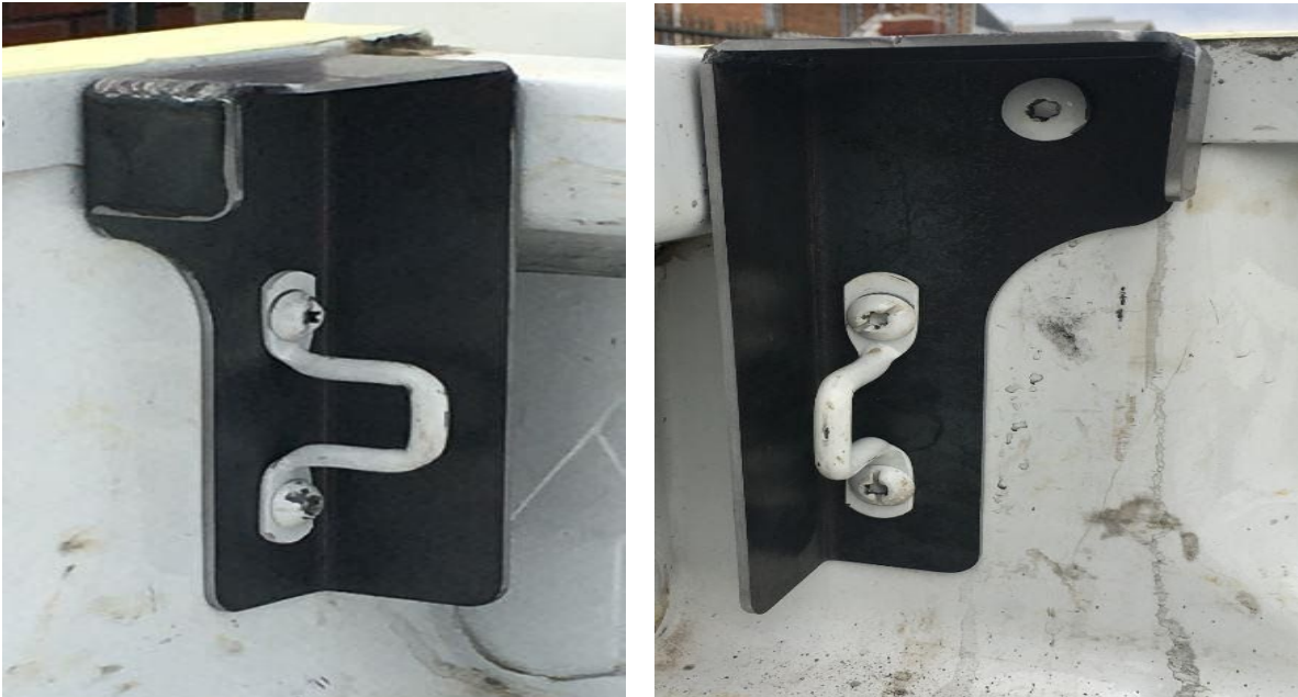
Figure 12: Front Bracket installed
