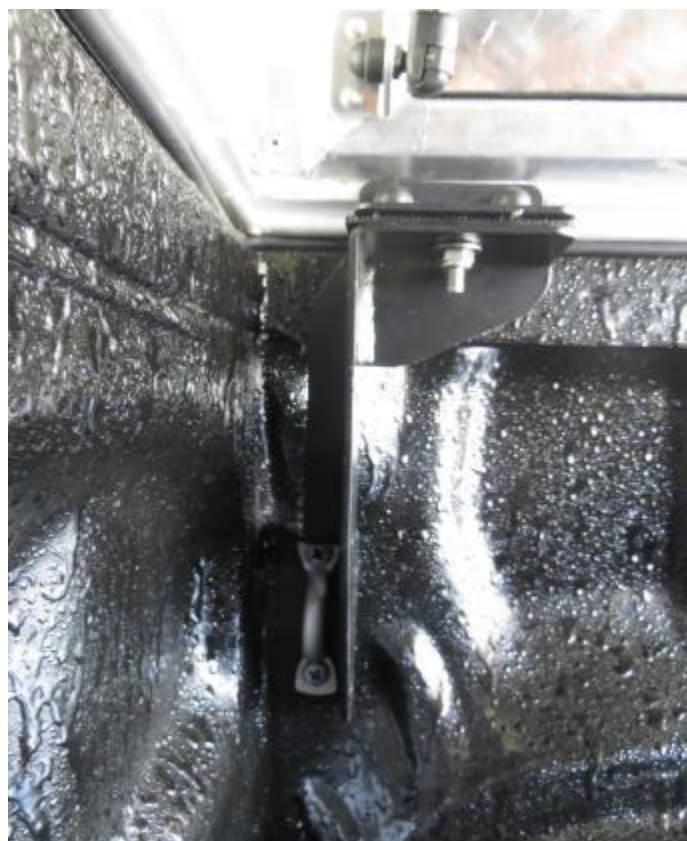
Figure 21: Front-Right Support Bracket Installed
