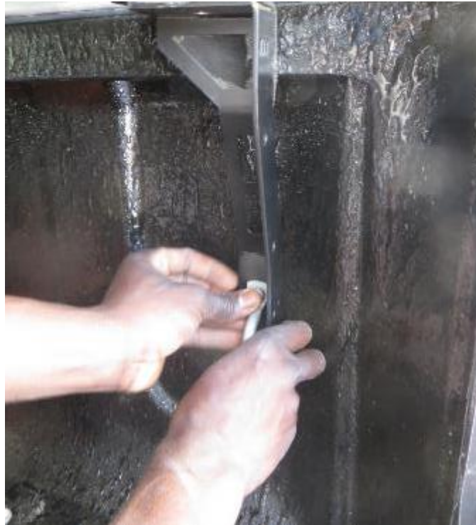
Figure 8: Aligning the Rear Support Bracket
