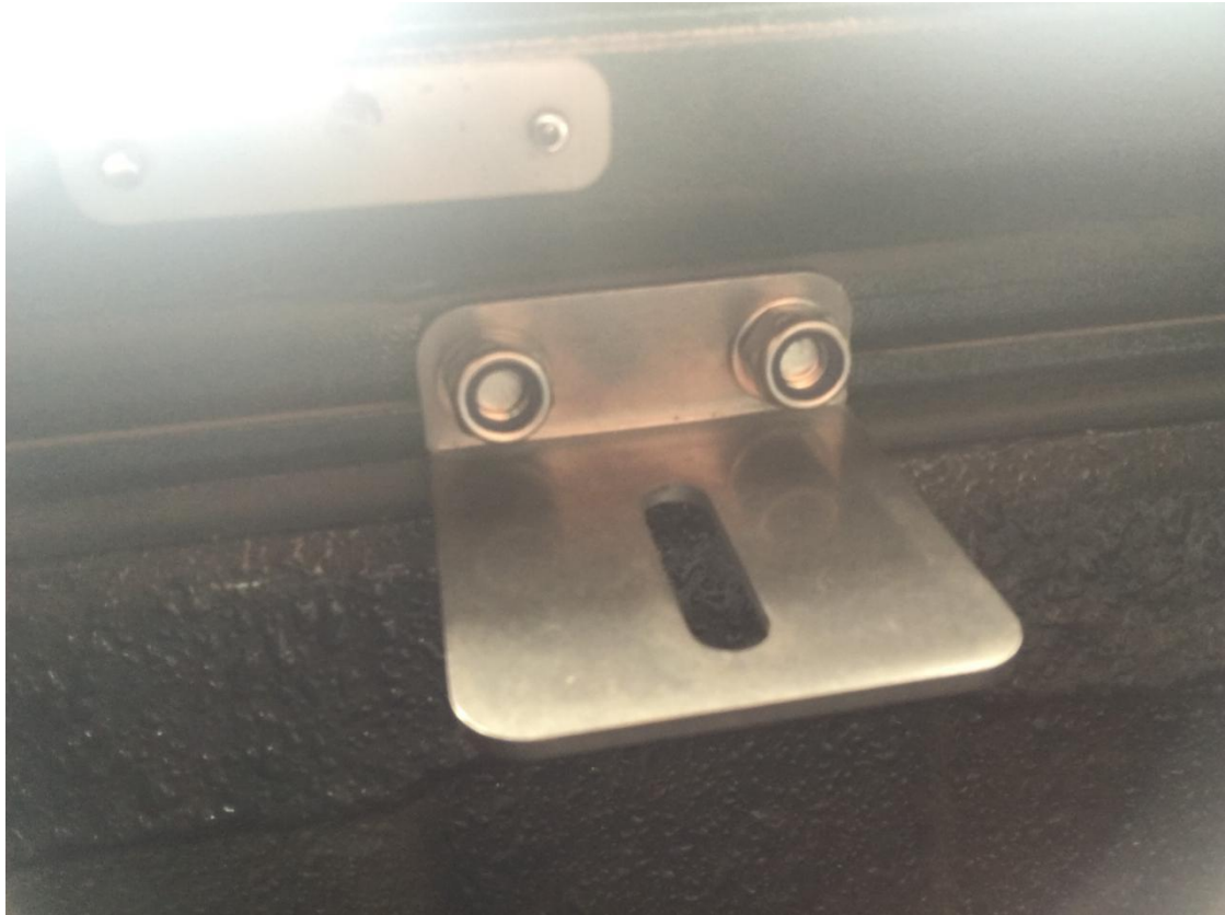
Figure 8: Finger Tighten Nyloc Nuts onto the Bolts
