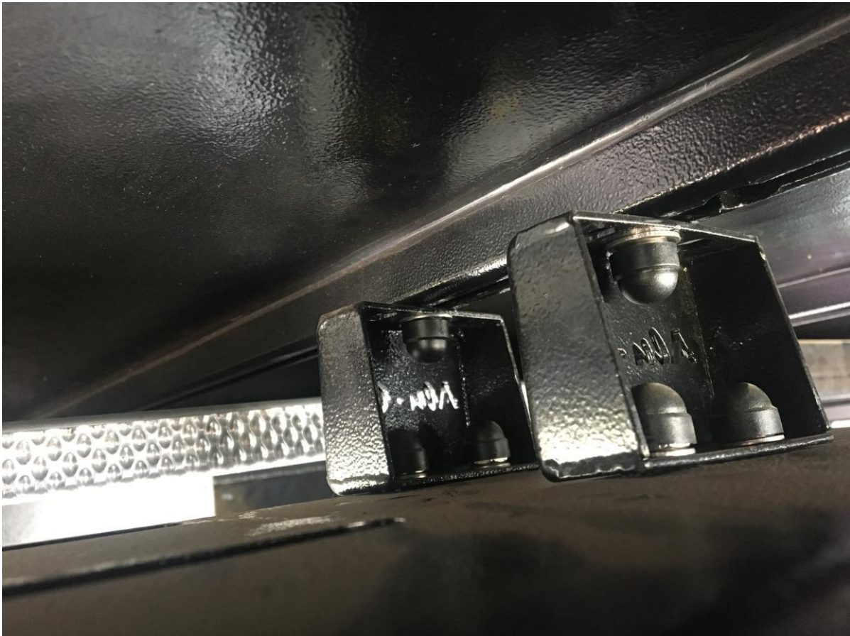
Figure 13: Place Nut Caps on the exposed Nuts
