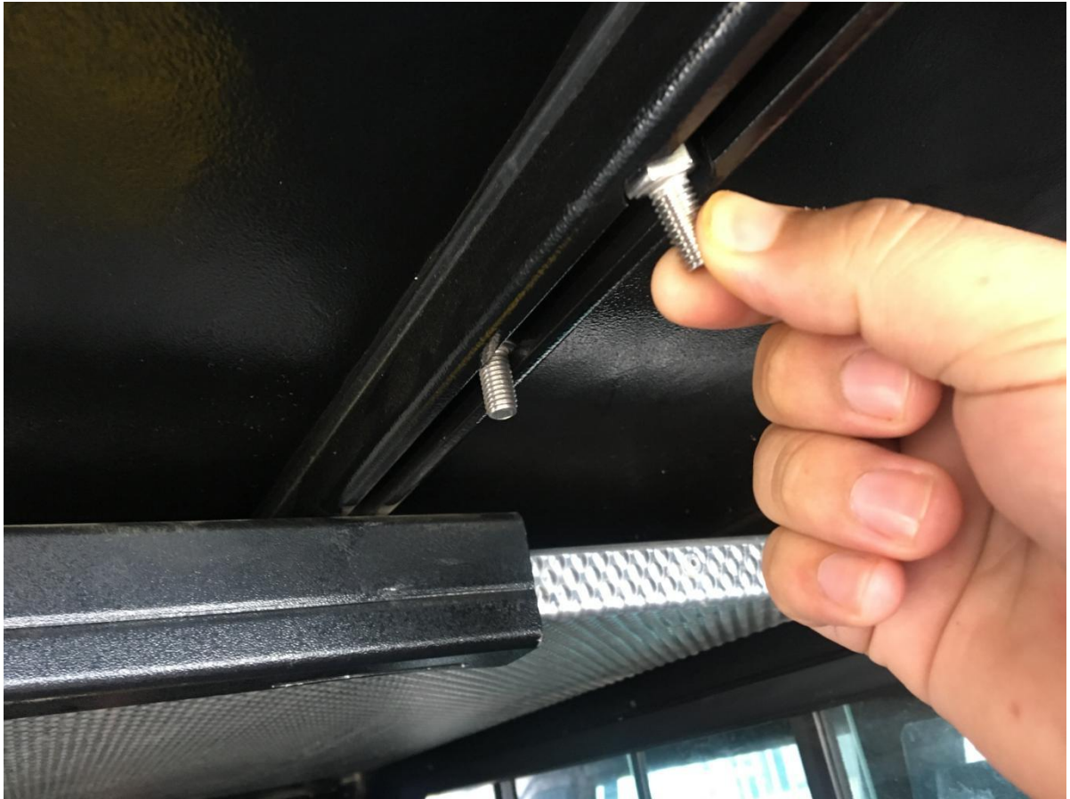
Figure 1: Inserting Hex Bolts into roof Nut Slot
