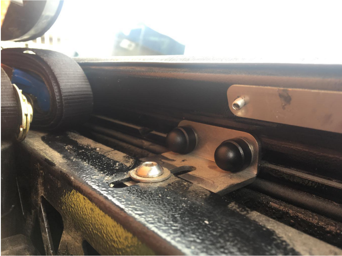
Figure 17: Side Mounting Completed with Nut Caps
