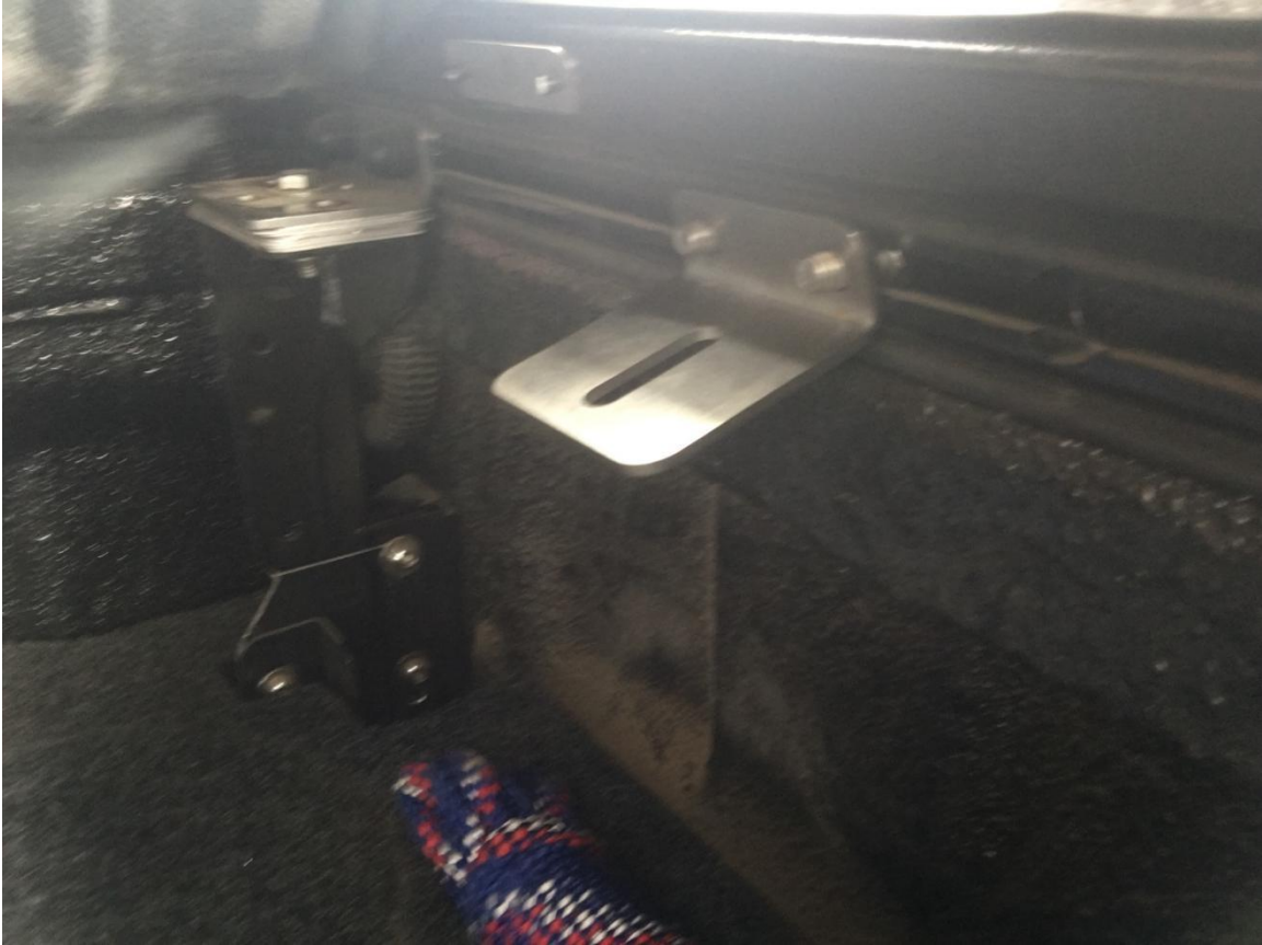
Figure 6: Canopy Side Nut Slot and Mounting Bracket
